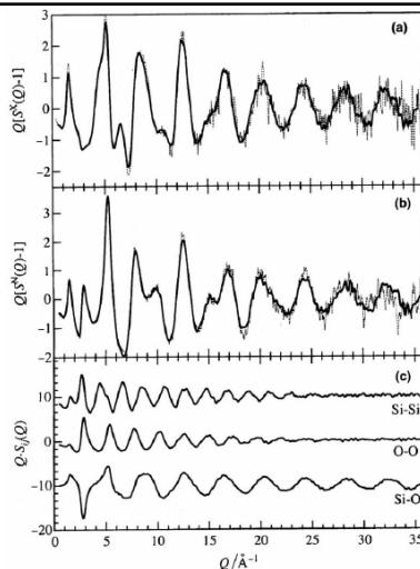
Figure 6. Reverse Monte Carlo simulation of silica glass compared to high-energy X-ray scattering (a) and neutron scattering (b). The interference functions,  $Q(S(Q)-1)$  differ because of the different cross-section weightings. Dashed lines are experimental and solid lines the result of RMC modelling. The partial structure factors for Si-Si, O-O and Si-O obtained from RMC modelling are given in (c), displaced vertically. Reproduced with permission from [60]. © 2001 Elsevier.
