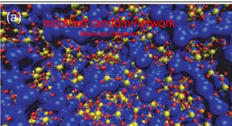
Figure 19. Static alkali channels modelled with molecular dynamics in alkali silicate glasses. (a) 'Snapshot' of the structure of the  $\text{Na}_2\text{Si}_3\text{O}_7$  glass silicate with the Na atoms (blue) emphasized with an enlarged equipotential isosurface. Reproduced with permission from Meyer *et al.* Meyer, J., Horbach, W., Kob, F., Kargl and H. Schobler, Phys. Rev. Lett. **93** 027801, 1-4 (2004).
