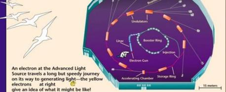
An electron at the Advanced Light Source travels a long but speedy journey on its way to generating light—the yellow electrons at right give an idea of what it might be like! The text and pictures around the edge of the poster will help you follow the action inside the ALS, beginning with the electron gun. Whenever you see the key symbol  $e^-$ , you can find more explanation in the Key Concepts section below.
